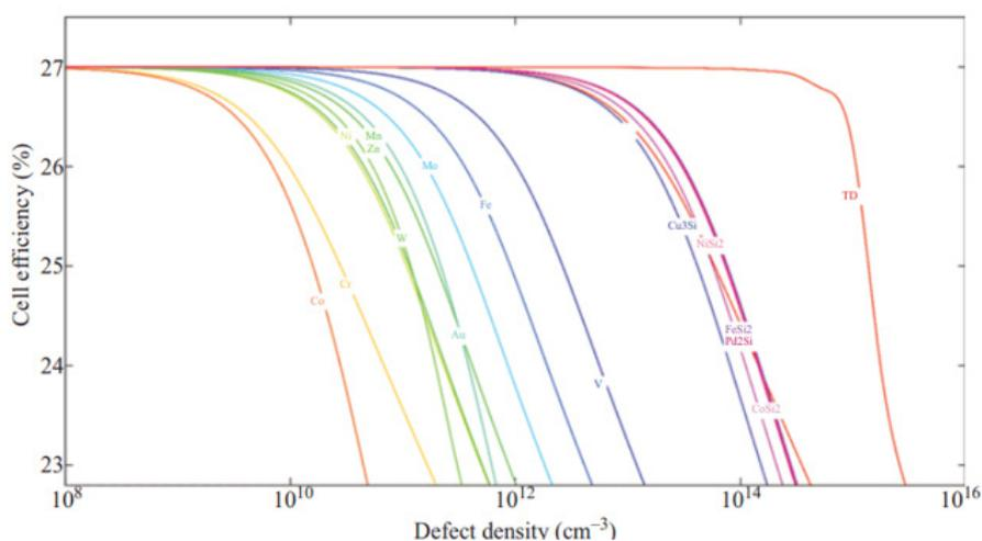
Figure 2. Cell efficiency in relation to the number of impurity defects[12].
