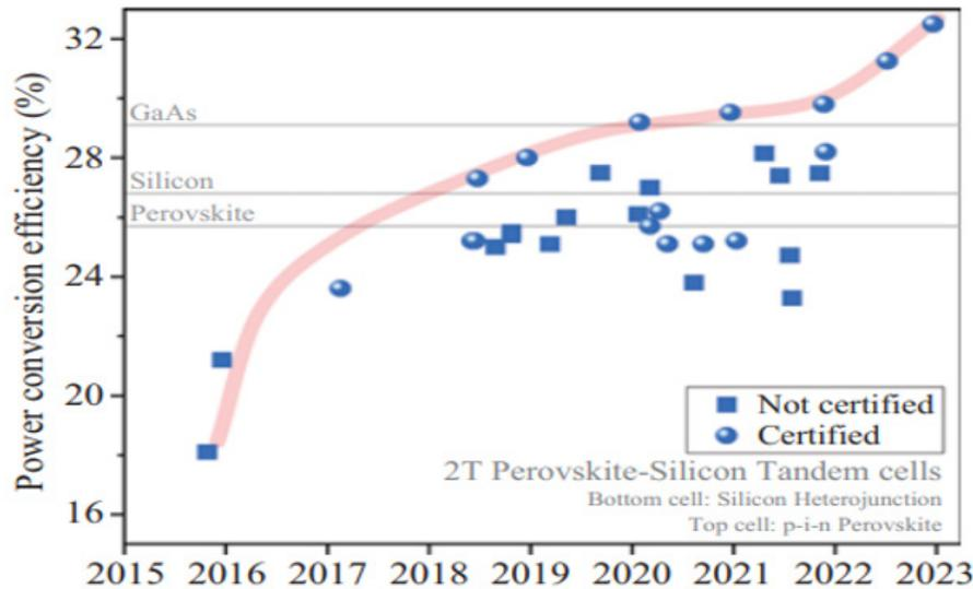
Figure 9. The study demonstrates the highest power conversion efficiencies of two-terminal perovskite-silicon tandem solar cells, surpassing the record efficiencies of other single junction technologies under the global AM1.5 spectrum.
