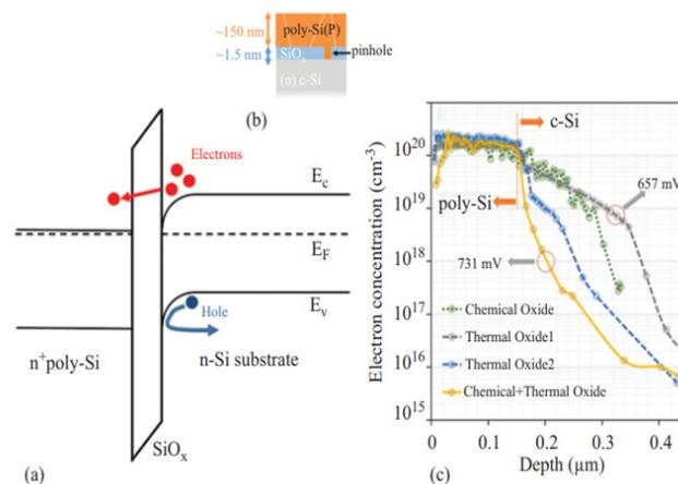
Figure 5. The study presents a schematic band diagram and electron concentration profiles of a poly-Si(n+)/ $SiO_x$  passivated contact, highlighting the influence of the  $SiO_x$  layer on dopant diffusion into the c-Si substrate and its effect on surface passivation level [7], [12].
