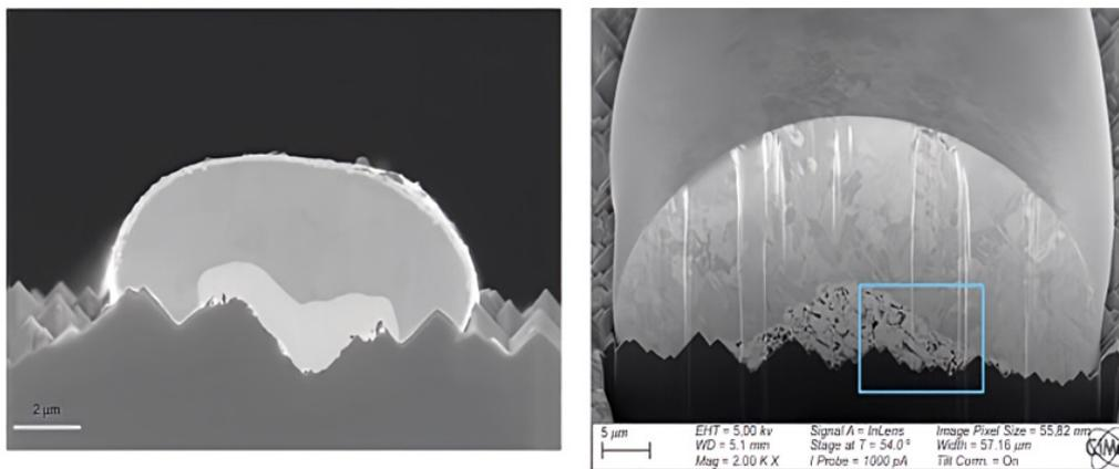
Figure 7. Cu-plated finger cross-sectional pictures taken using a scanning electron microscope. Left: A Topcon solar cell with fingers plated in Ni, Cu, and Ag. Right: A screen-printed Ag seed-grid application with a Cu-plated finger [40], [41].
