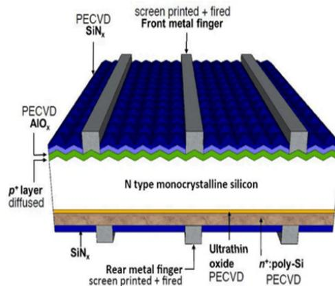
Figure 1. A schematic image of an n-Si solar cell with a description of its different layers [5].
