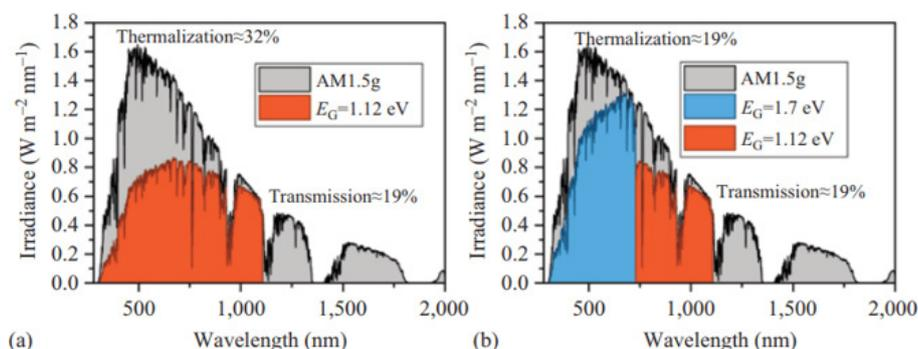
Figure 8. The AM1.5g spectrum fraction can be used in single-junction solar cells with 1.12 eV bandgaps like silicon or combined with materials with 1.7 eV and 1.12 eV bandgaps. In tandem solar cells, high energy photons absorb in the top cell, reducing thermalization losses to 19%[55].
