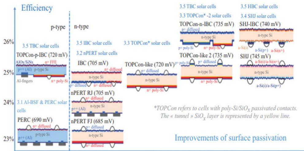
Figure 4. Diagrammatic illustrations of the many solar cell technologies discussed in this chapter. The advances in surface passivation are represented by the x-axis. With respect to the conversion efficiency, the y-axis [12].
