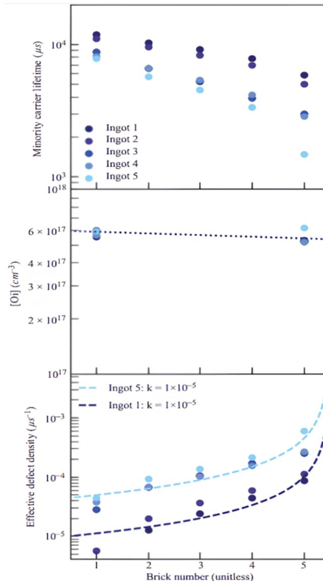
Figure 3. shows the effective defect density, interstitial oxygen concentration, and minority carrier lifespan in an n-type ingot after five recharges[12].
