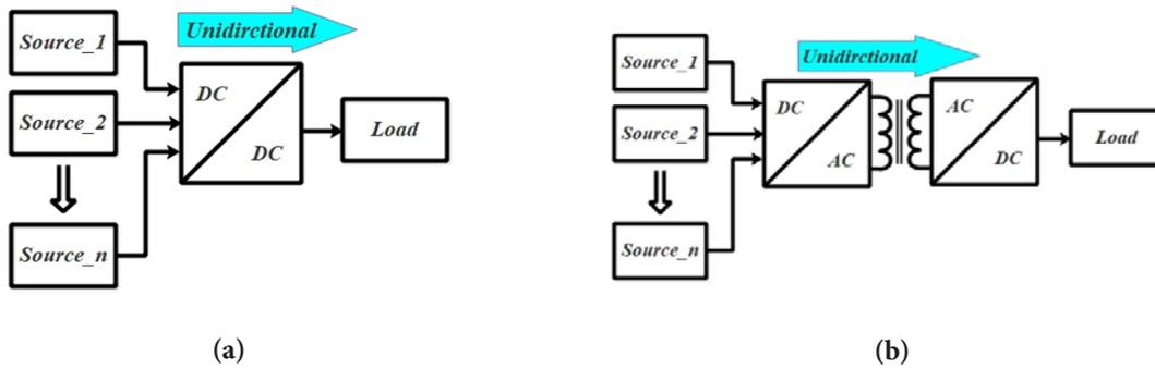
Figure 2. (a) Unidirectional non-isolated MPC & (b) unidirectional isolated MPC.
