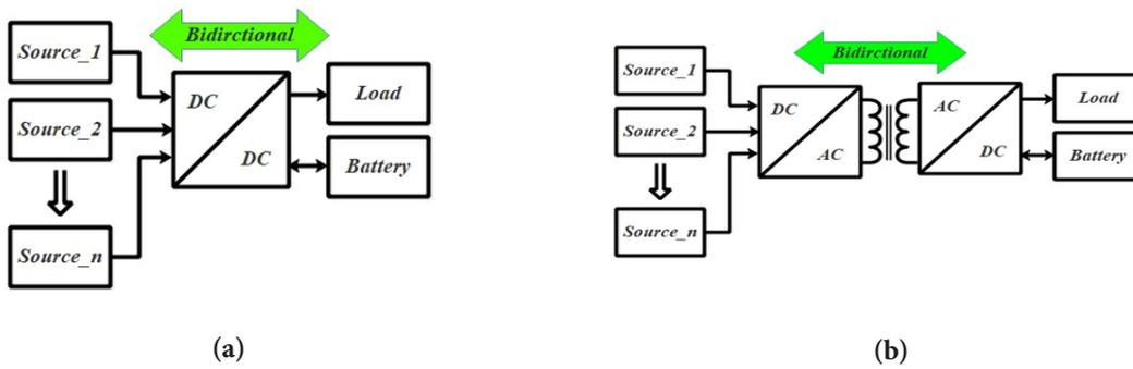
Figure 3. (a) Bidirectional non-isolated MPC & (b) Bidirectional isolated MPC.
