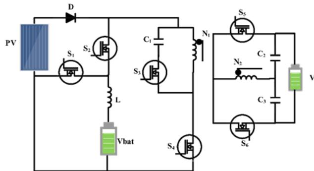
Figure 6. Circuit diagram of three-port bidirectional converter in [114].
