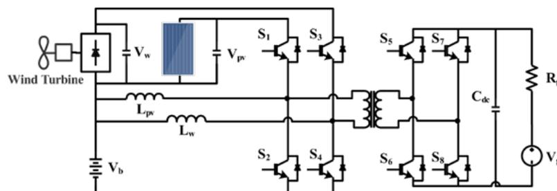
Figure 11. Circuit diagram of the Presented MPC in [132].
