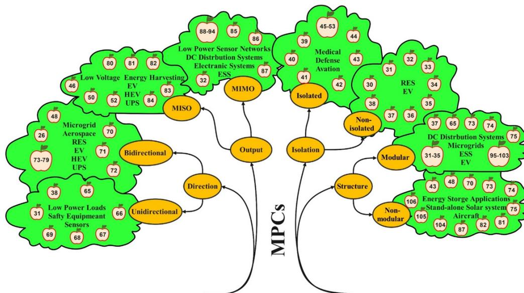
Figure 1. The general classification of MPCs based on Applications.
