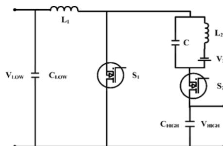
Figure 9. Circuit diagram of the Presented MPC in [123].
