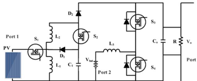
Figure 8. Circuit diagram of three-port bidirectional converter in [121].
