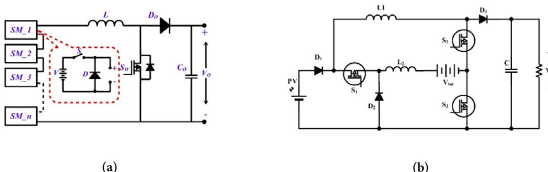
Figure 4. (a) Basic structure of MISO and (b) MIMO converter.
