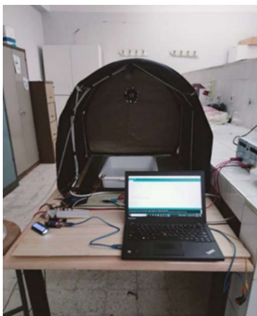
Figure 1. Overview of the Smart Greenhouse Controlled by Arduino.
