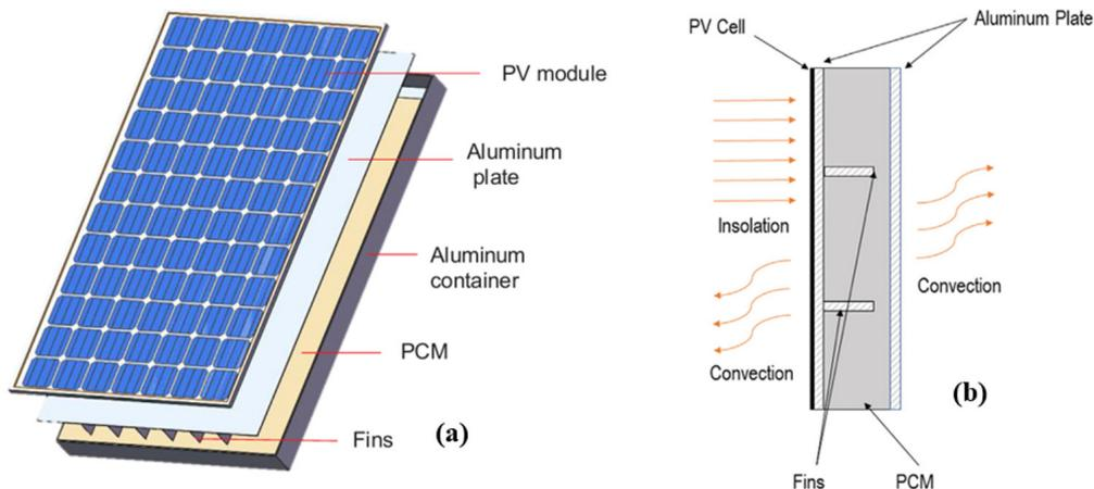
Figure 18: (a) 3-D view of the PV/PCM module; and (b) Cross-sectional view of the PV/PCM module [129].
