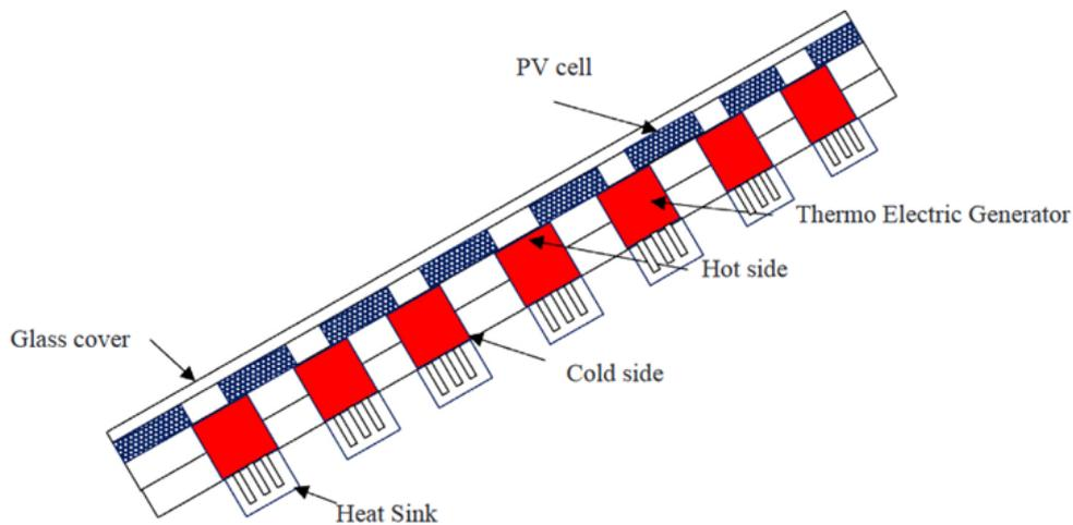
Figure 12: Cross-sectional view of the PV-TE module [86].
