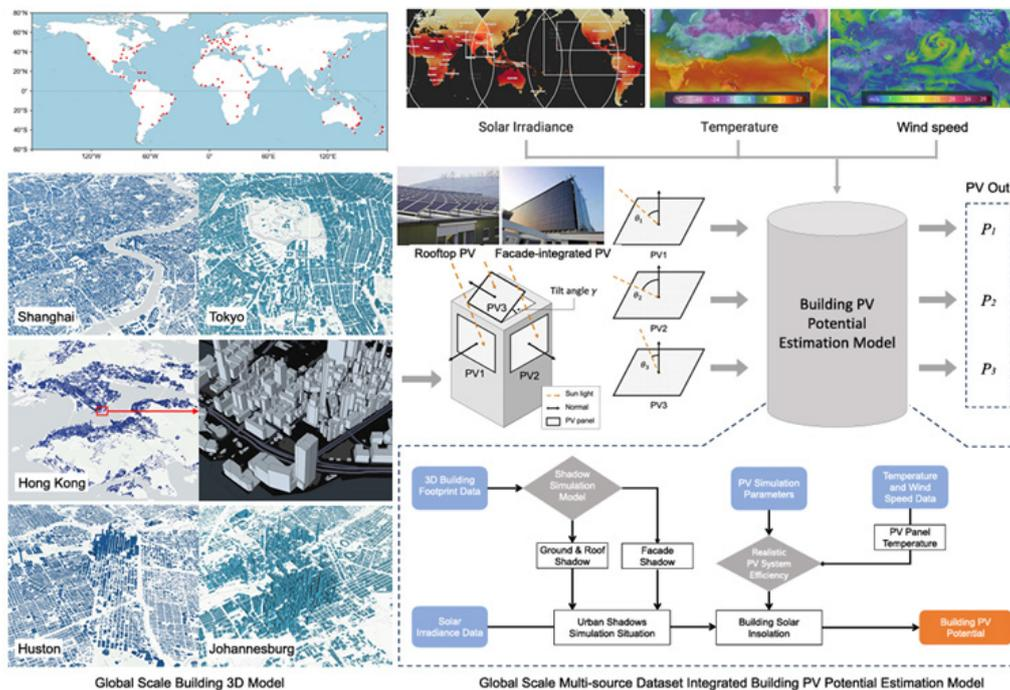
Figure 14: Framework for estimating the photovoltaic potential of building façades and roofs worldwide [109].
