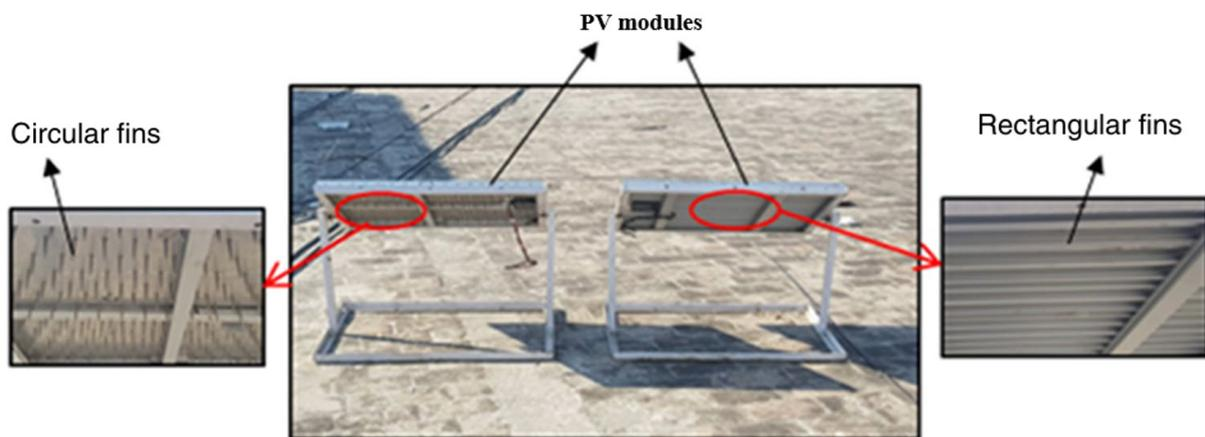
Figure 6: Experimental setup illustrating the arrangement of fins with PV modules [37].
