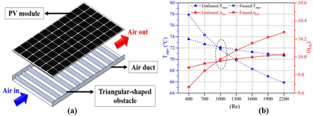
Figure 15: (a) Air hybrid PVT collector with triangular obstacles [115]; and (b) Effect of the increase in temperature of the PV module on electrical efficiency in different ranges of Reynolds number for air hybrid PVT collectors with and without fins [123].
