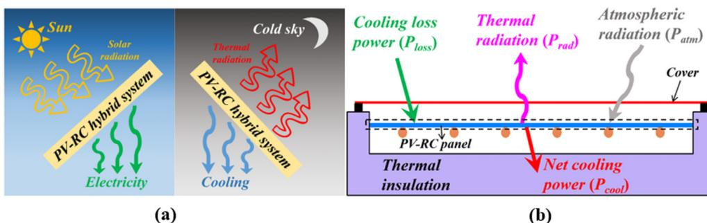
Figure 9: (a) Concept for using a radiative-cooled PV module; and (b) Radiated PV module thermal analysis diagram [79].
