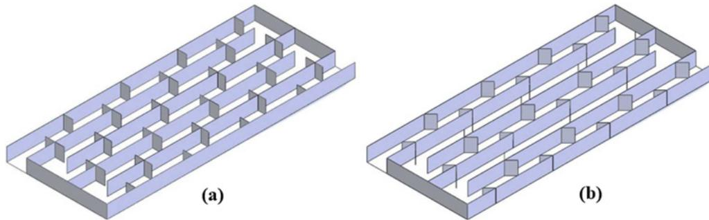
Figure 19: (a) Channel with fin coupling and T-shaped baffles; and (b) Channel with fin coupling and V-shaped baffles [128].
