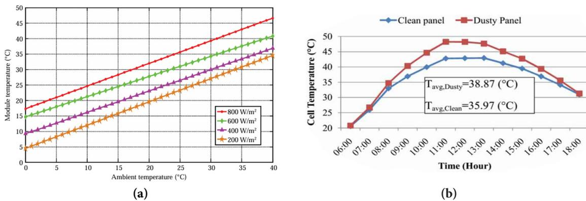
Figure 4: PV module temperature: (a) as a function of ambient temperature at different levels of solar radiation; and (b) dusty and clean panels PV [17].
