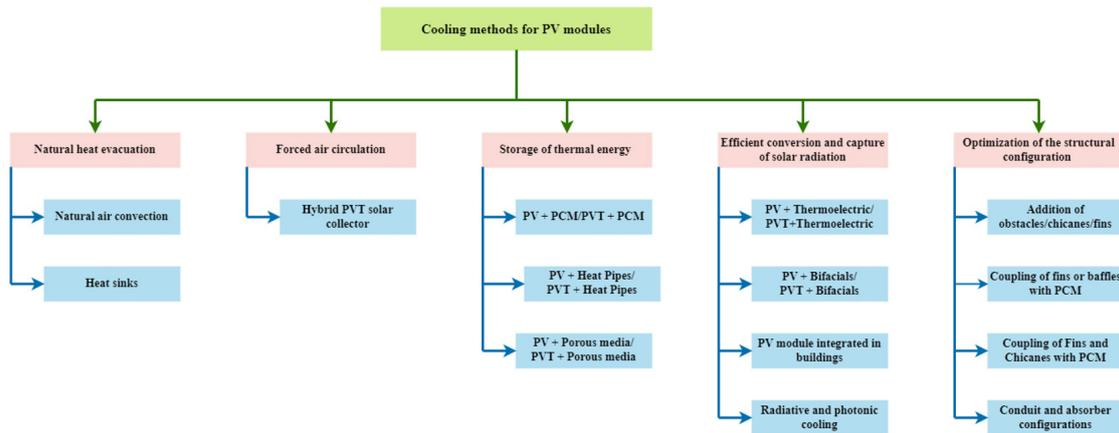
Figure 5: Classification of cooling methods for PV modules.
