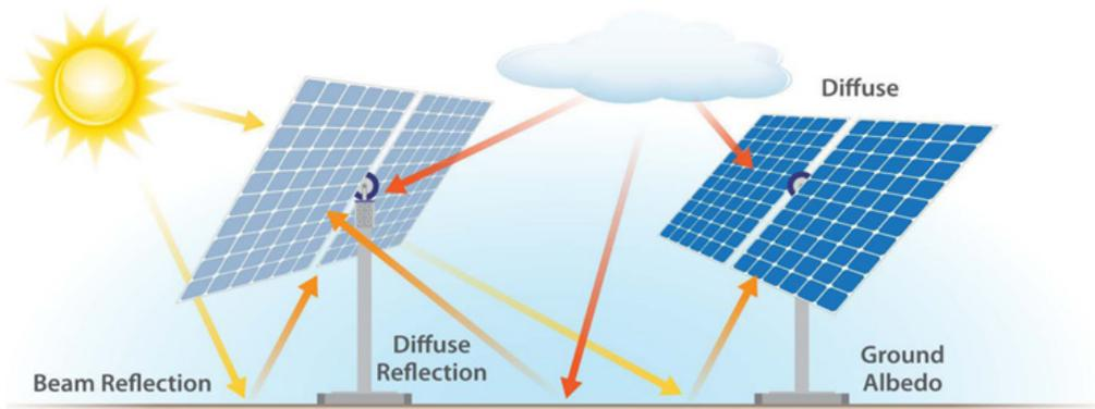
Figure 13: Illustration of the operation of a bifacial PV module [110].
