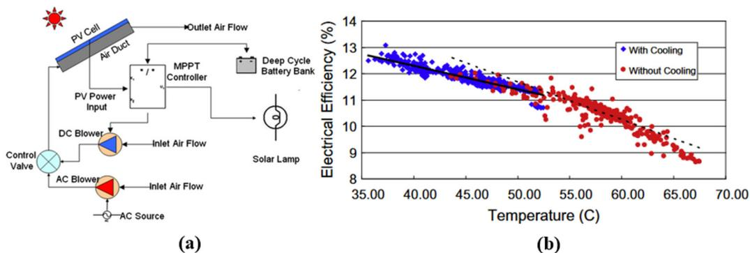
Figure 7: (a) Experimental set-up for forced air circulation in ac hybrid PVT collector; and (b) Electrical efficiency as a function of PV module temperature [19].
