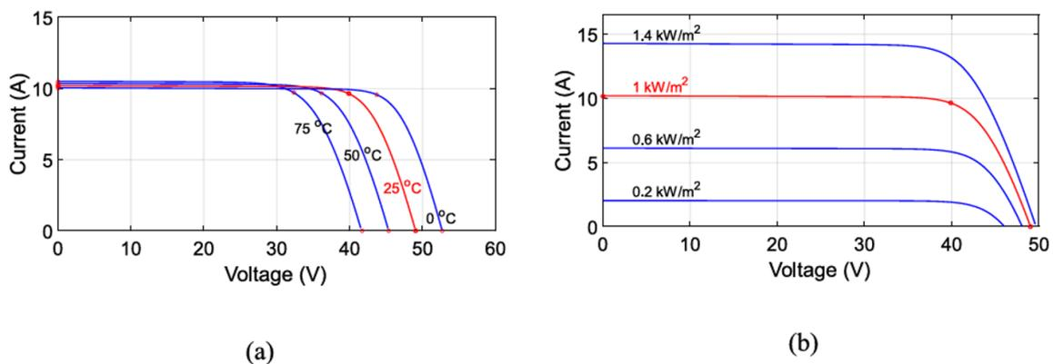
Figure 2: PV module current-voltage curves: (a) Variable PV module temperature; and (b) Variable solar irradiance [27].
