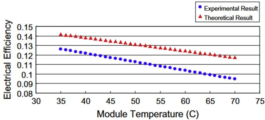
Figure 3: Electrical efficiency as a function of PV module temperature [28].
