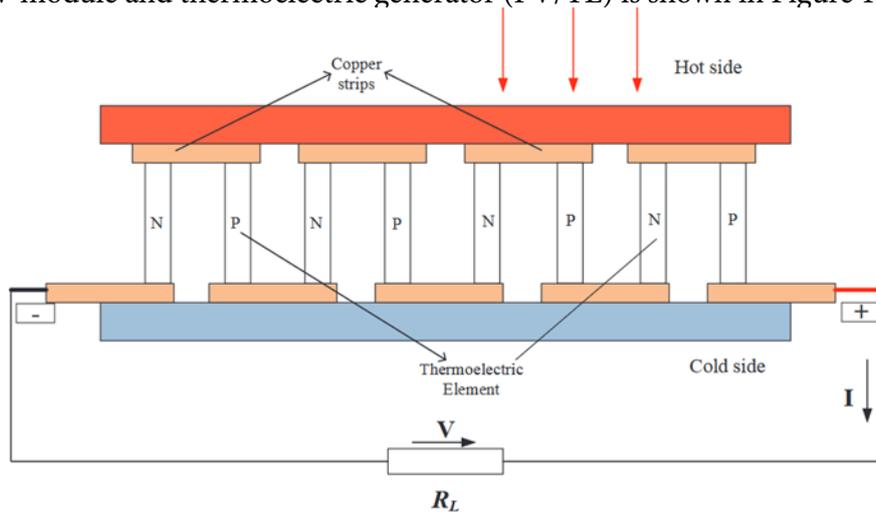
Figure 11: Basic thermoelectric generator structure [86].
