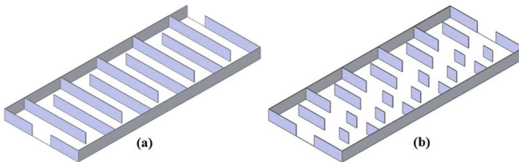
Figure 16: (a) single fin channel; and (b) multiple fin channel [128].
