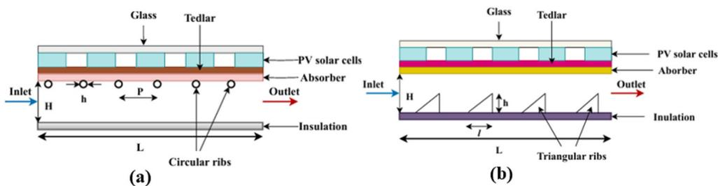
Figure 17: (a) Configuration of the circular ribs under the PV module [126]; and (b) geometric configuration with triangular ribs [127].
