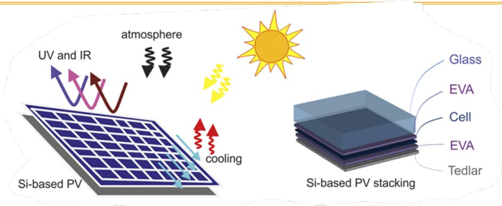
Figure 10: Schematic of cooling approaches for radiative and photonic thermal management of PV modules and stacking of crystalline silicon-based encapsulated PV module materials [80].
