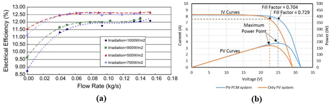
Figure 8: (a) Influence of air mass flow on efficiency [28]; and (b) PV/PCM and standard PV module current-voltage and power-voltage curves [56].
