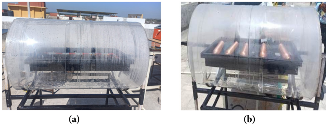
Figure 2. (a) & (b) Conventional Tubular solar still without pcm & Modified Tubular solar still with copper bottles with inserted copper hollow tubes Conventional Tubular solar still without pcm.
