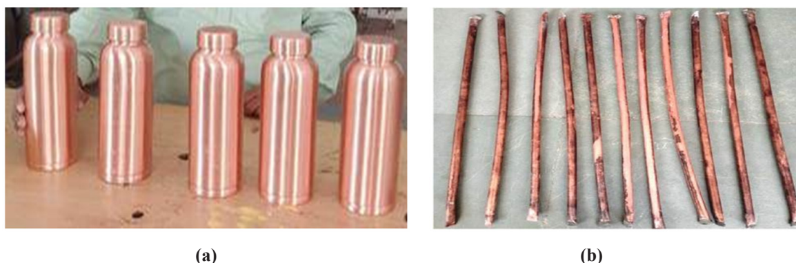
Figure 1. (a) Copper bottles with PCM filling; and (b) Copper hollow tubes.
