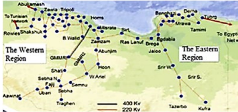
Figure 2. High-Voltage Transmission Network in Libya [26].
