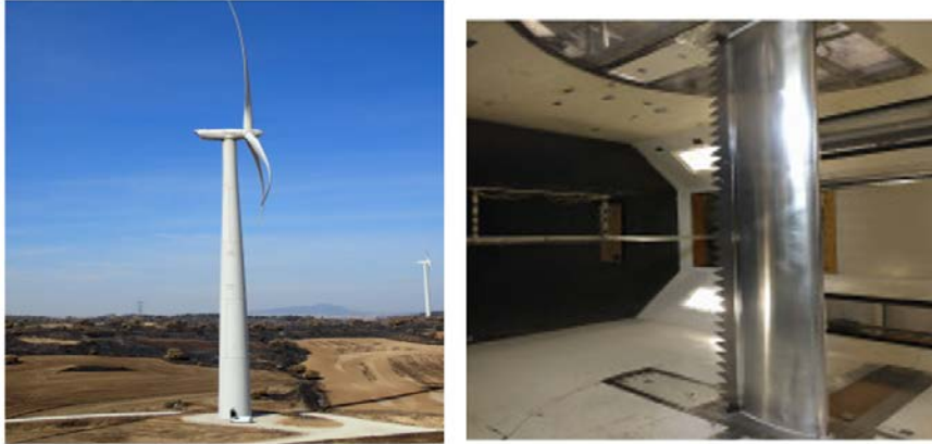
Figure 8 NACA64s418 model implemented in the studied wind turbine (on the left) [98].
