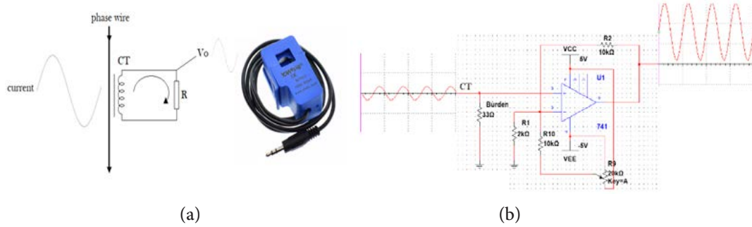
Figure 7: (a) current transformer, (b) Amplification circuit on 2.5 volts dc level.
