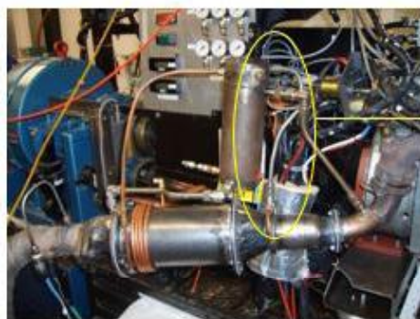
Figure (1b). The integrated reformer connected to V6 engine
